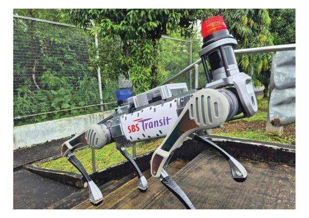
LiDAR technology, high-definition cameras, thermal imaging and video analytics to detect intrusions or signs of tampering more accurately than its human counterparts. This allows officers to focus on higher-level tasks. The pilot results have been promising, paving the way for MARS to be deployed at additional depots.
